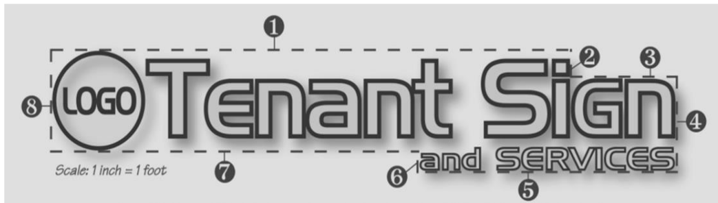
Example of eight-line measurement of a sign
